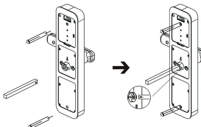
Take the front panel, fix the handle shaft to the lock, align it with the latch to stabilize it. It is not easy to fall off. And fix the screw sleeve onto the upper and lower screw posts.
