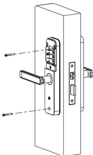
Remove the rear panel, insert it into the handle shaft, align it with the screw hole on the panel, open the battery cover, and secure the last two panel screws
