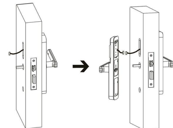
Align the square axis on the front panel with the lock hole and thread it through, and also thread the wire head and screw sleeve through the door hole.
