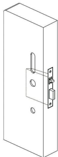
Place the lock body into the door slot of the opened hole and secure it with two lock body screws
