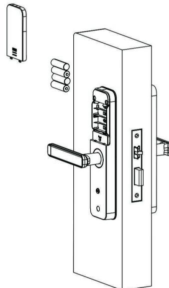
Insert the battery and cover it with the battery cover. After installation, enter the initial password to verify unlocking, and use the mechanical key to unlock for
